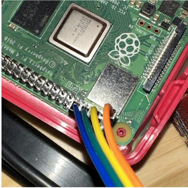
On the Raspberry Pi's GPIO header, these correspond to pins 1, 10, 8, and 6. The numbering and relative placement of these pins are the same on all (non-pico) Pi, including the original Raspberry Pi with the shorter GPIO header and Pi Zero models.
